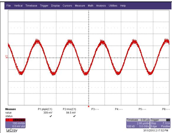
Typical Output Ripple at Vin,nom and Full Load at Ta=25C
