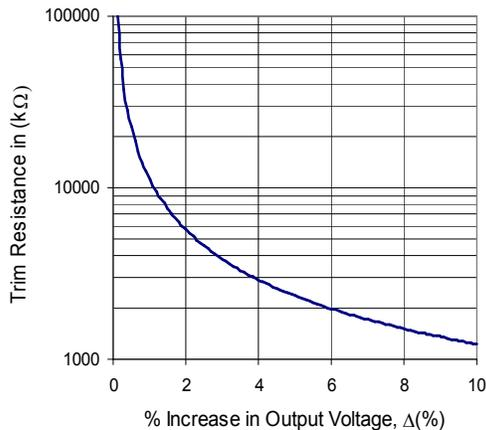
The value of Vref can be found in the Electrical Data section of this data sheet. The maximum power available from the power module is fixed. As the output voltage is trimmed up, the maximum output current must be decreased to maintain the maximum rated power of the module. It is also desirable to slightly increase the input voltage while trimming up the output with heavy load current.
