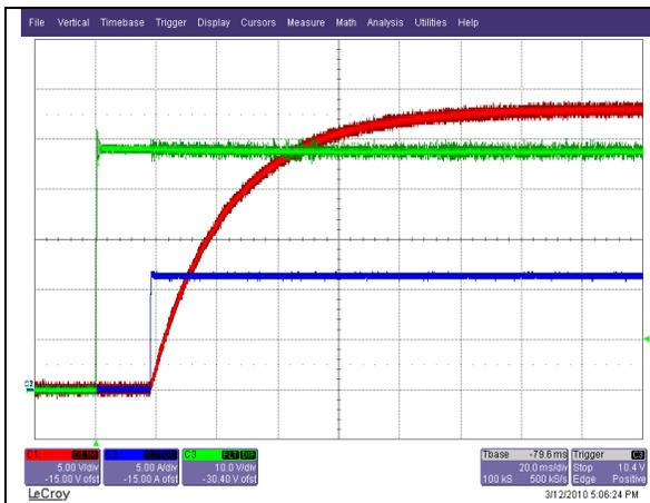
Start-up from Input Voltage Application at Full Load.
